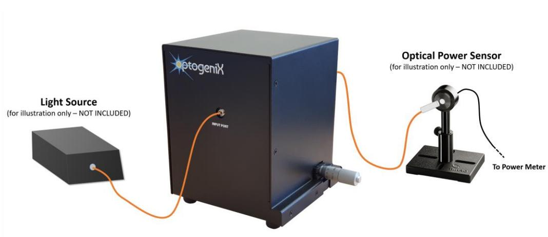
**Figure 5** Setup for optical power calibration
